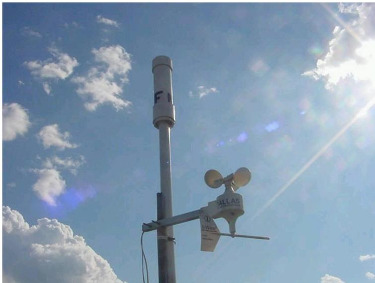
The mast is 1 ½ inch PVC while the container for the detector is 3 inch PVC mounted to a tripod on the roof.
